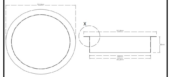
Materials: Constructed from Type UK 304 stainless steel, 0.9mm gauge with exposed surfaces in a Black Matt Finish
