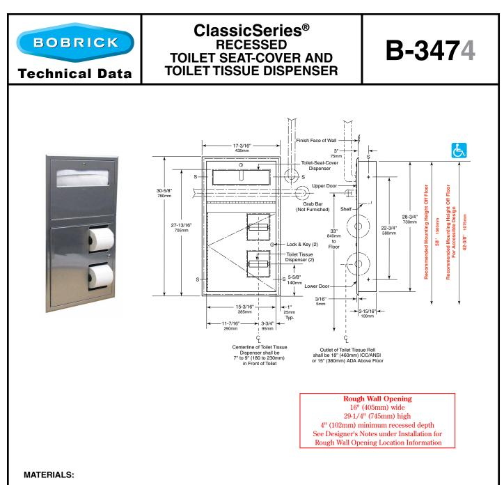
Cabinet — 18-8, Type-304, heavy-gauge stainless steel. All-welded construction. Exposed surfaces have satin finish.
