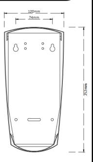
Materials: Constructed from type 304 stainless steel exposed surfaces are polished finish.
