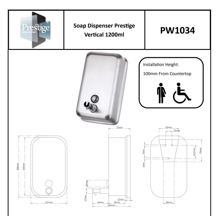
Materials: Constructed from type 304 stainless steel, exposed surfaces are in a brushed finish.
