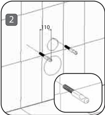
2. Screw on the two metal fixings on the threaded bar of the frame.
