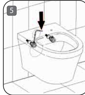
5. When you put the Pan on the threaded bars make sure that the fixings don't move and remain secure.
