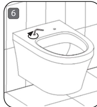
6. Adjust the Pan and secure it with the fixing nuts through the seat holes in the top of the Pan. An allen key is supplied.
