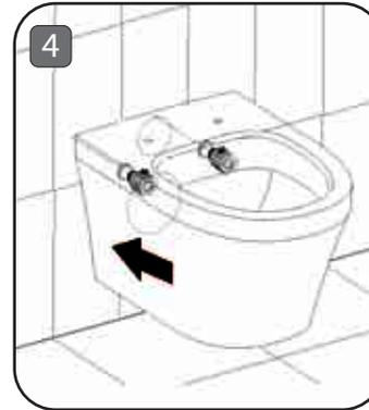
4. Then place the Pan onto the threaded bars and push it until flush to the wall, taking care of the connections which must be perfectly engaged to each other.
