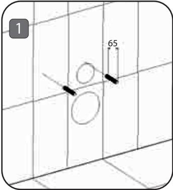
1. Prepare the waste and the fixing rods as shown in the picture and cut if necessary
