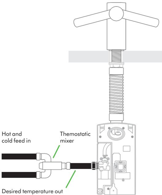
If connecting to cold only water feed you will need to install a heater.
