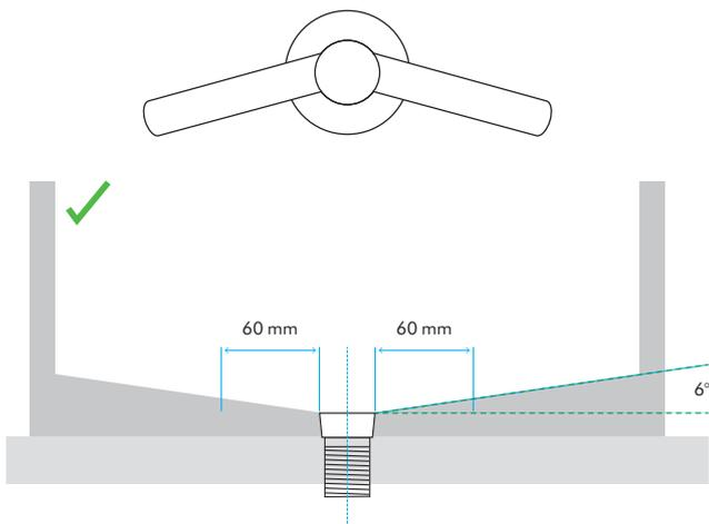
Minimum of 6° ramp angle from the edge of the drain hole of the sink will result in good drainage leading to reduced levels of splashback (minimum 60 mm radius).
