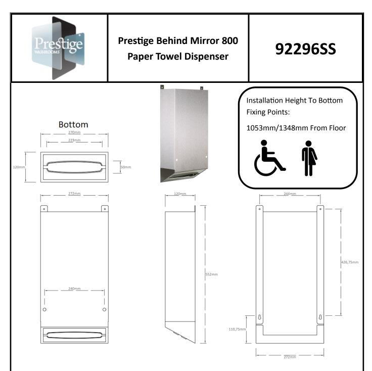
Materials: Constructed from high quality stainless steel, exposed surfaces brushed finish.
