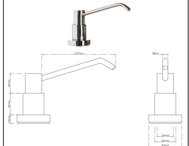
Materials: Constructed from chrome plated brass with exposed surfaces in a polished finish.
