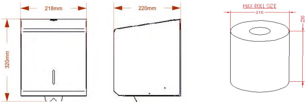
Height: 320mm Width: 218mm Depth: 220mm Weight: 3.4Kg Capacity: 210mm Standard C/feed Roll
