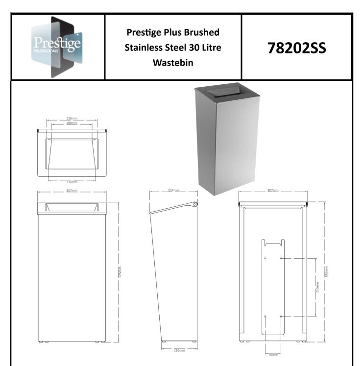
Materials: Constructed from type 304 stainless steel exposed surfaces are brushed finish.
