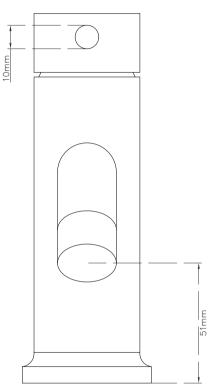
Counter hole Ø 28-40mm Maximum counter thickness 40mm
