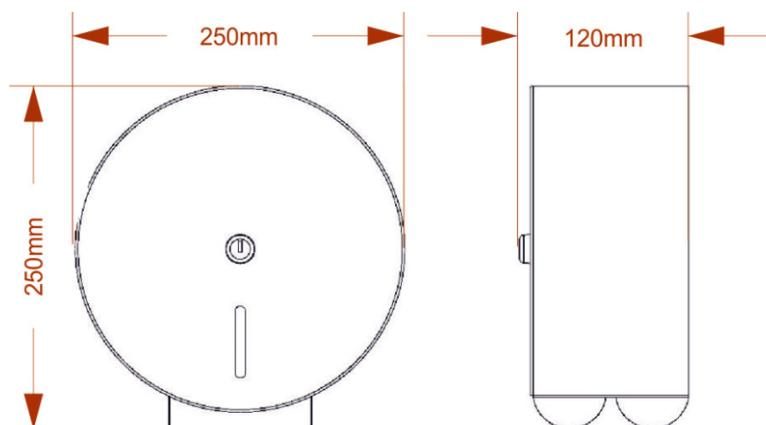
Height: 250mm Width: 250mm Depth: 120mm Weight: 1.7Kg Capacity: 250mm Roll
