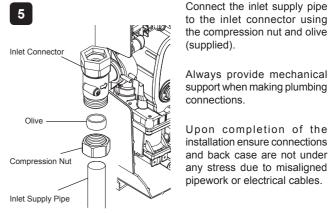
the compression nut and olive (supplied). Always provide mechanical
