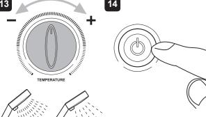
Adjust temperature as required. Push START/STOP button. Light Flow rate will adjust automatically. in the button goes out.
