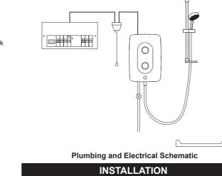
Warning! Isolate the electrical and water supplies before installing the shower
