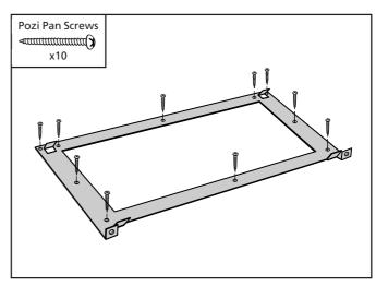
Secure frame using the 10 gauge x 20mm screws provided.
