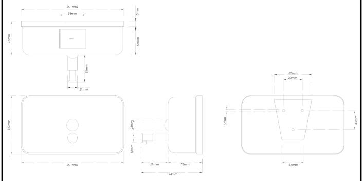
Materials: Constructed from type 304 stainless steel, exposed surfaces are in a brushed finish.
