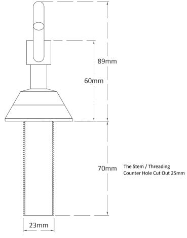
Dimensions: Above Counter 60mm. Under Counter 250mm Available in 2 spout lengths: 100mm & 127mm, see options. Chrome plated on solid brass body The piston is removable for convenient refilling from above counter top Spout - high quality stainless steel High quality non-drip pump Spout will not rotate
