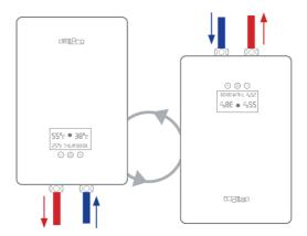
NOTE The temperature display will reamin in a fixed position regardless of mounting position.
