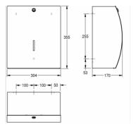
Jumbo toilet roll holder for wall mounting, stainless steel, surface satin finished, front with InoxPlus surface refinement for the reduction of finger marks and better cleaning characteristics (easy to clean), material thickness 1.5 mm, closed casing with curved front, paper withdrawal over two tear-off edges, cylinder lock with Franke standard key, for 1 roll with max. Ø 295 mm, incl. stainless steel screws and dowels.
