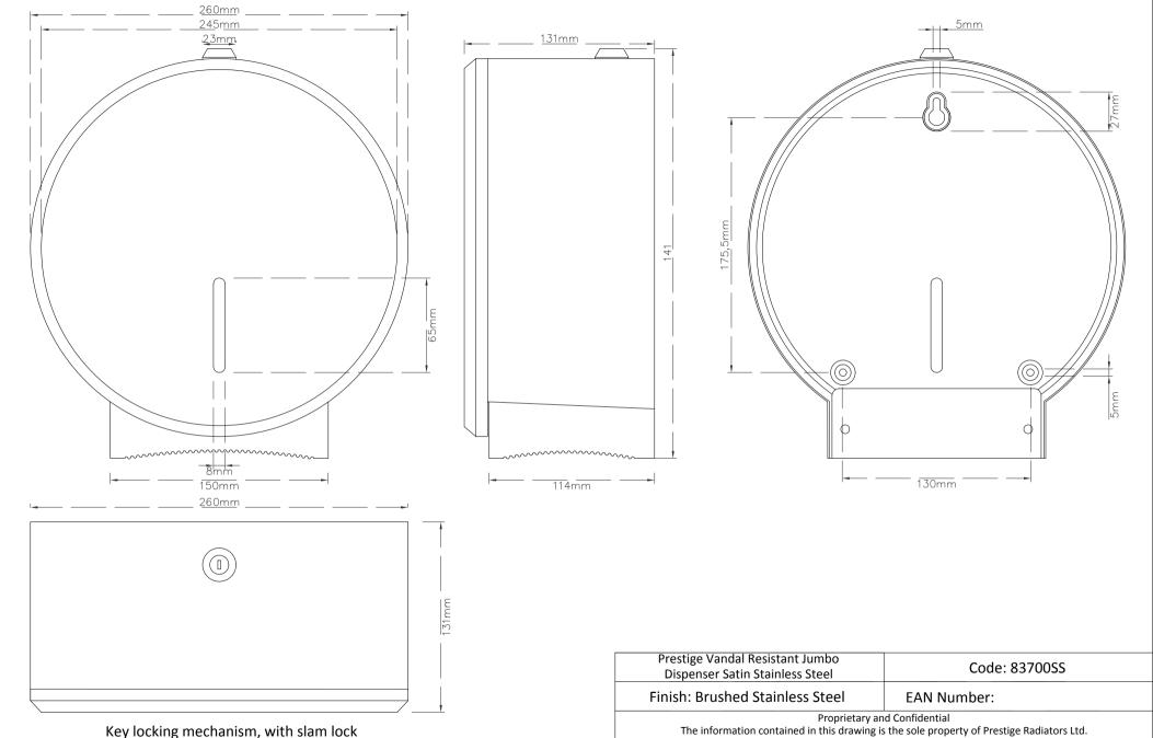
Capacity: Core Dia 45mm, Max Roll 315mm, Width 98mm Core Dia 57mm, Max Roll 330mm, Width 98mm Core Dia 76mm, Max Roll 320mm, Width 98mm
