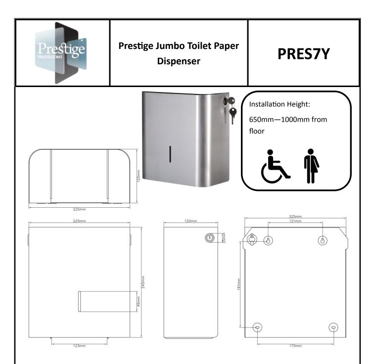
Materials: Constructed from type 304 stainless steel, exposed surfaces brushed finish.
