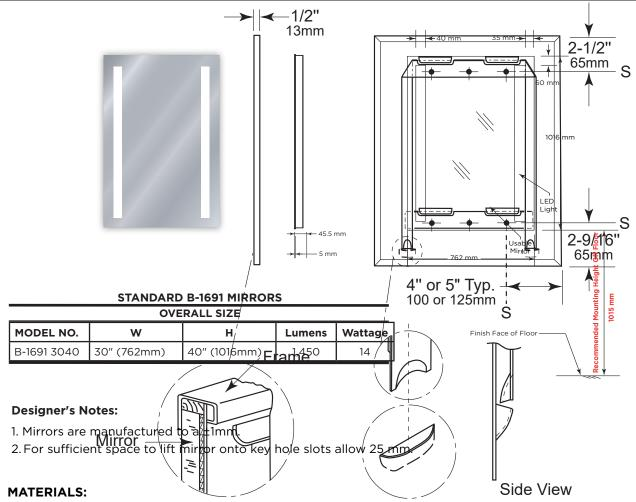
Glass — 5 mm thick safety mirror with 0.14 mm PVC film backer with free safety safety Hanger Extruded Back — Aluminium channel with mounting holes.
