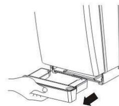
2. Remove drain tank and empty.
