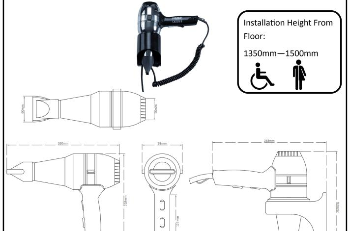
Materials: Constructed from stainless steel and ABS.
